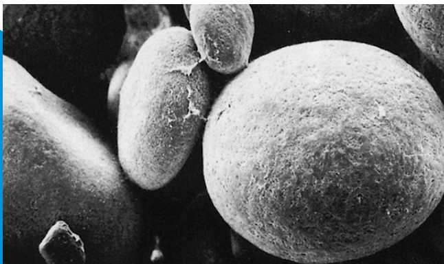
Contact tartrate after having used contact crystals for several months in red wine stabilization; separation by hydrocyclone.
