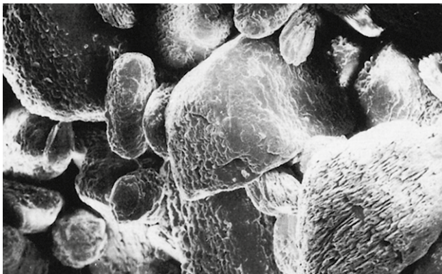
Contact tartrate after fourth re-usage in white wine stabilization; separation by hydrocyclone.
